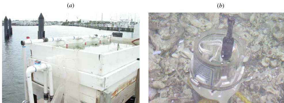
Figure 6. (a) Photograph of the raceway filled with seawater from Bayboro Harbor. (b) Photograph of the PCB MEMS CTD submerged in the raceway. The black extension is a communication connector plug.
